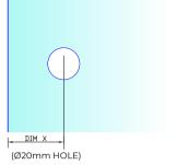
DIM X = 27mm + DIM (t) (GLASS THICKNESS)
